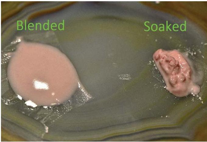
**Figure 3:** The porcelain masses (blended and soaked) immediately after mixing.
