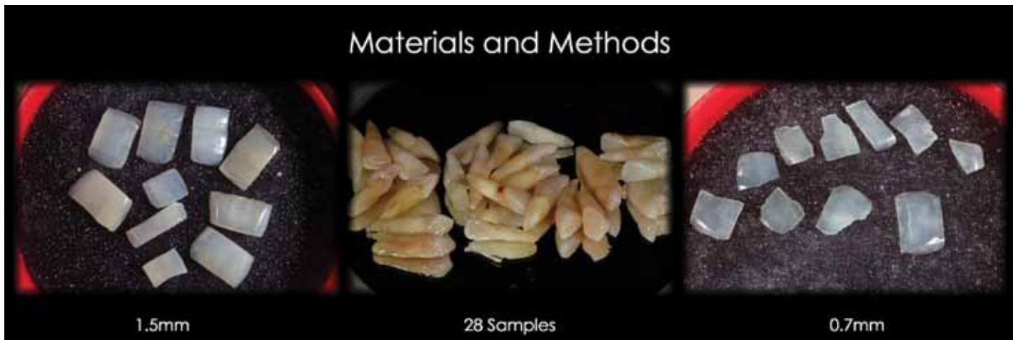
Figure 6: The enamel from 28 natural teeth was carefully removed into slices, each with a thickness of 0.7 mm, to replicate the size and thickness of a porcelain laminate veneer.
