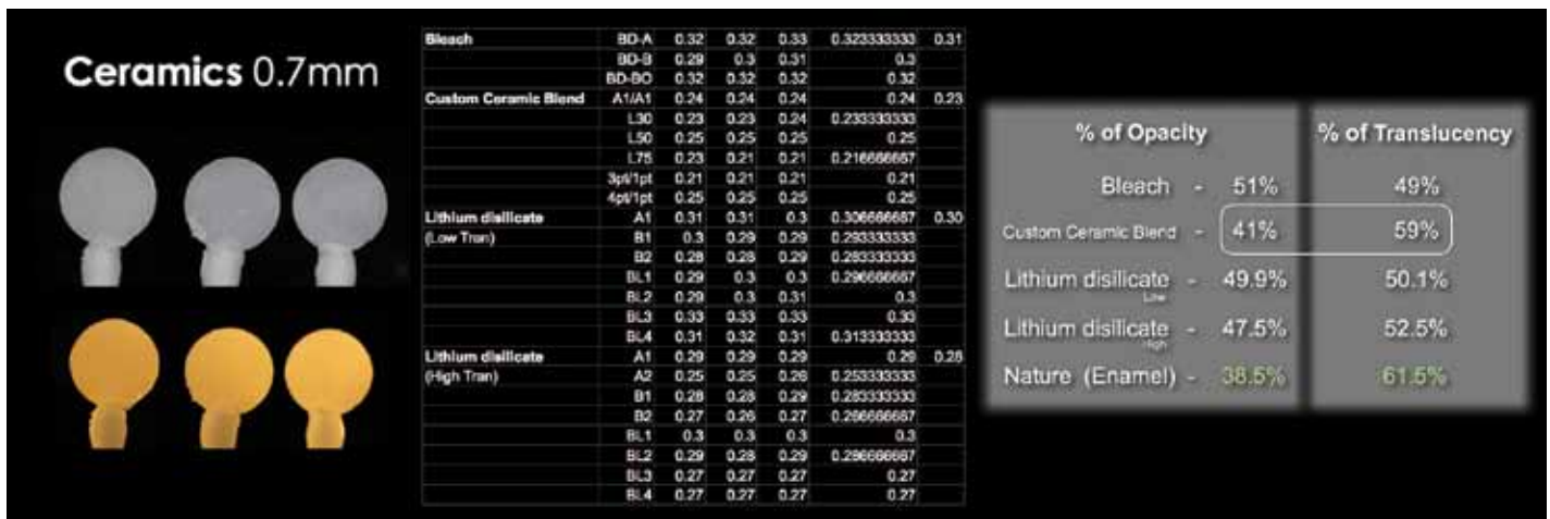
Figure 9: The off-the-shelf ceramics were up to 21% less translucent compared to that of natural enamel, whereas the author’s customized blend was much closer to natural enamel, with a difference of only 5%.
