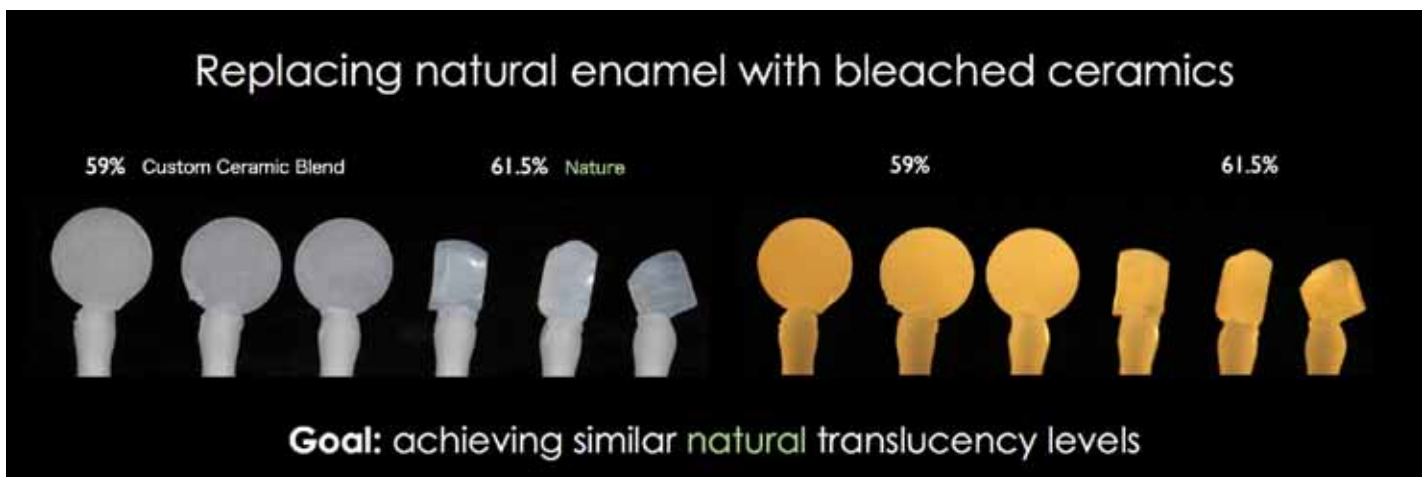
Figure 10: When replacing natural enamel with bleached ceramics, the goal is to achieve translucency levels as close to natural enamel as possible.
